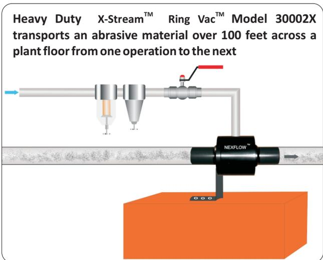
Heavy Duty X-Stream™ Ring Vac™ Model 30002X transports an abrasive material over 100 feet across a plant floor from one operation to the next
